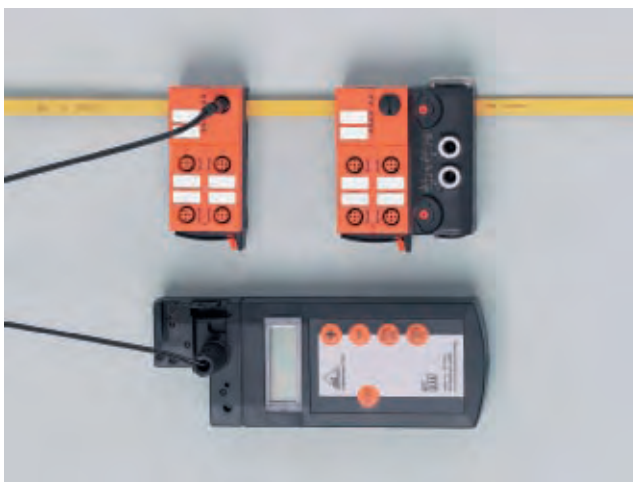
Convenient addressing of the ClassicLine modules via the the addressing socket.
