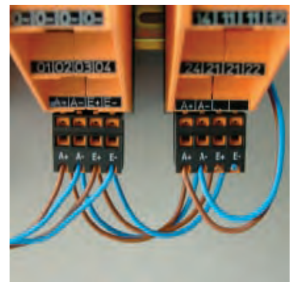
QUIX wiring allows replace- ment of modules during operation.
