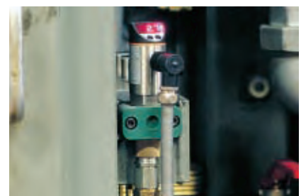
Analogue value detection of system pressure.
