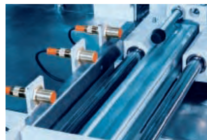
Inductive sensors on a traversing slide.
