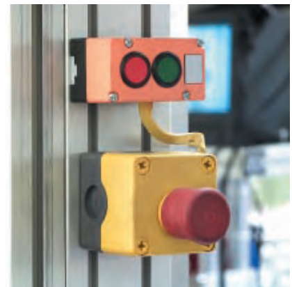
Intelligent AS-i slave: Emergency stop switch.
