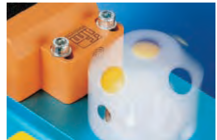
Easy as ABC: Puck with two metal targets offset by 90° and inductive dual sensor for position detection of the shaft.
