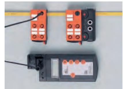
Using the addressing unit the slaves can be easily programmed via cable.
