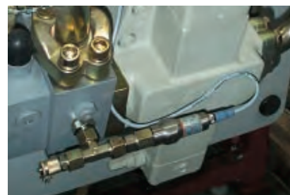
AS-i pressure sensors on a valve unit.
