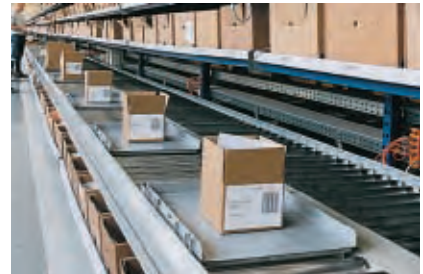
In the ifm logistics centre in Essen all sensors in the conveyor are connected to the higher-level controller via AS-i.
