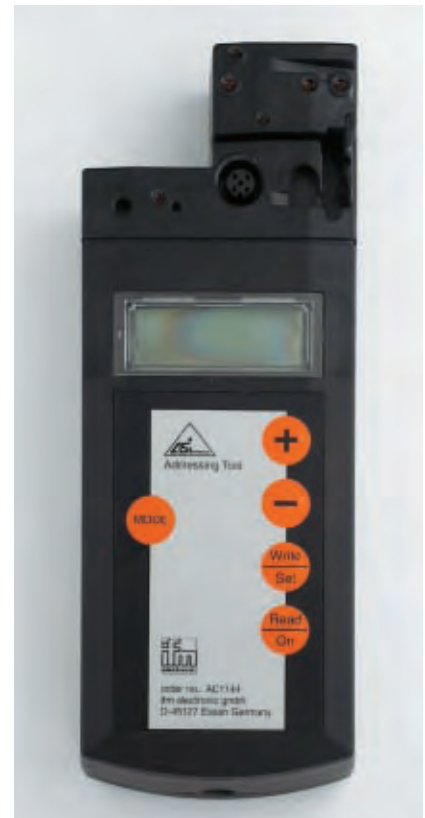
AS-i addressing unit for diagnostics and set-up.
